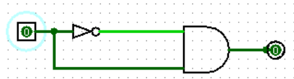
Fig.10: ENAND gate Ladder Mode Output – Input OFF
